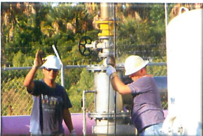
Mechanical Integrity Test of our injection well.
